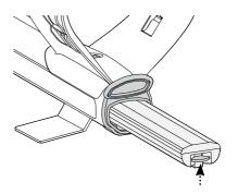
**5** Remove the battery pack entirely from the battery compartment.
