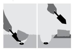
Check the hole for the target. If it is not in the hole, place the detector on the ground with the coil flat, pick up a handful of soil and pass it over the coil. Be sure not to wear rings, bracelets or a watch which will produce a signal. Repeat this procedure until the target is located.
